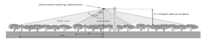
**Fig. 1.** Representation of limits of the areas corresponding to the field of view (FOV) contributing to 50 and 90% of total signal for a downward looking radiometer with 180° FOV and cosine response.
